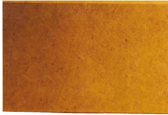
Fig. 6 Microstructure of failed tube (Ferrite only) (X200)
