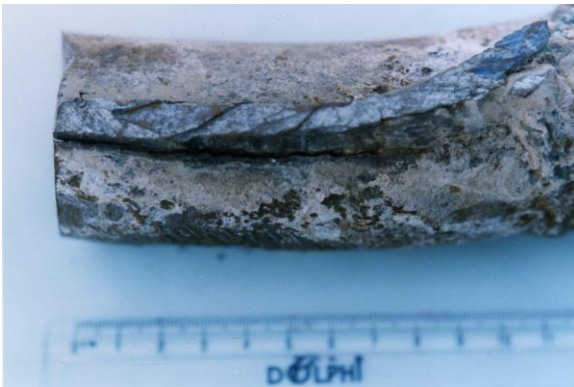
Fig. 3 Cracking in the tube
